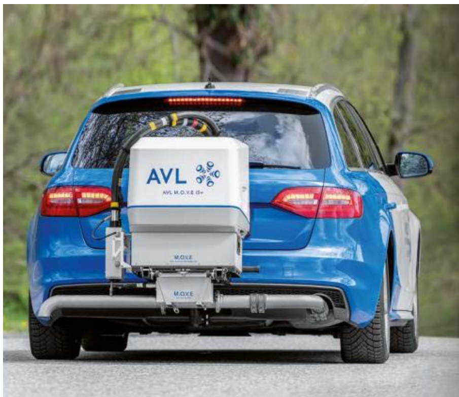
Figure 4 AVL PEMS equipment installed on the tow hook of a passenger car. Typical setup during a Real-Driving Emission (RDE) test
