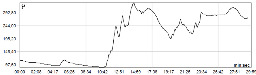
Figure 17: Exhaust temperature in °C measured before the SCR-system for the HDV 4 EURO V vehicle with a payload of 22 tons. The vehicle was driven on the highway. When the payload is added to the vehicle, the temperature in the exhaust system rises, indicating that the SCR-system becomes active due to the extra weight. The first 10 minutes is not part of the analysis because the vehicle drove around on the parking lot when being loaded.
